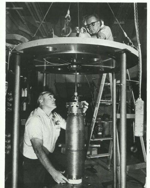
JOE BRADSHAW & HARRY OLSON (both 8413) adjust 8inch test unit before high speed spin test.
